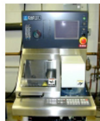
b) Computer-controlled dicing saw used for cutting wafers.
